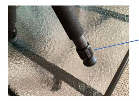
Extend tripod leg, as required, by undoing lock ring
